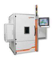
microCELL TLS laser system for half-cell cutting using thermal laser separation
