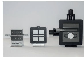
Sample fixtures with dovetail guide
