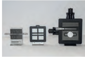
Sample fixtures with dovetail guide
