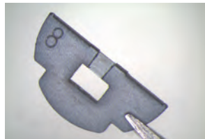
Basic structure cut and thinned (Photovoltaic Si-Wafer)
