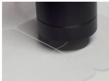
Process example: free form cutting of display coverglass
