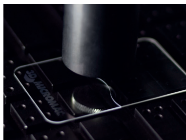
Process example: free form cutting of display coverglasses
