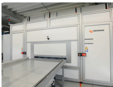
Example of handling table, fully automated substrate transfer into machine
