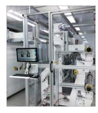
In flexible photovoltaics, 3D-Micromac's microFLEX™ PV systems are the perfect solution for laser structuring processes such as isolation cutting and ablation on front- or backside of thin-film substrates. The highly versatile systems can be completely customized to the individual process requirements. 3D-Micromac's expertise in the development of roll-to-roll machining solutions guarantees:
