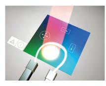
The microVEGA xMR uses on-the-fly spot and variable laser energy to provide selective heating of the pinning layer in each sensor in order to "imprint" the intended magnetic orientation.
